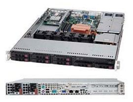
The SuperMicro 113 series case is a 1U chassis with 8 hot-swappable SAS/SATA bays and redundant power supplies. While requiring significant power for each quad core Xeon CPU, even 8 SATA Flash SSDs add only 16 watts to power consumption, producing a high performance system with around 270 watts of peak power consumption.
